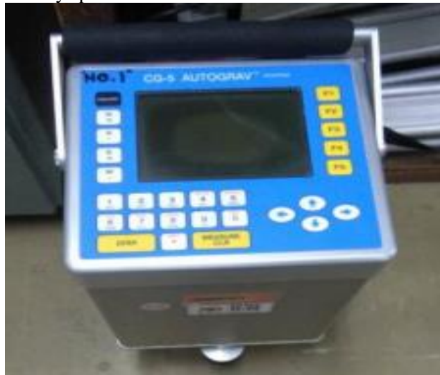
Figure 2: Equipment of the gravity measurements acquisition Scintrex CG-5 Autograv.
